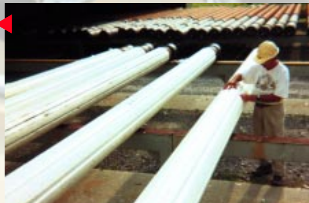
“Precision strength” syntactic foam has received industry recognition for engineering excellence in protecting highly pressurized well casings.
