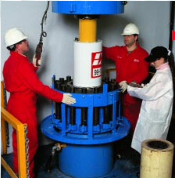
This custom-built simulated service vessel tests new material formulations for hydrostatic integrity.
