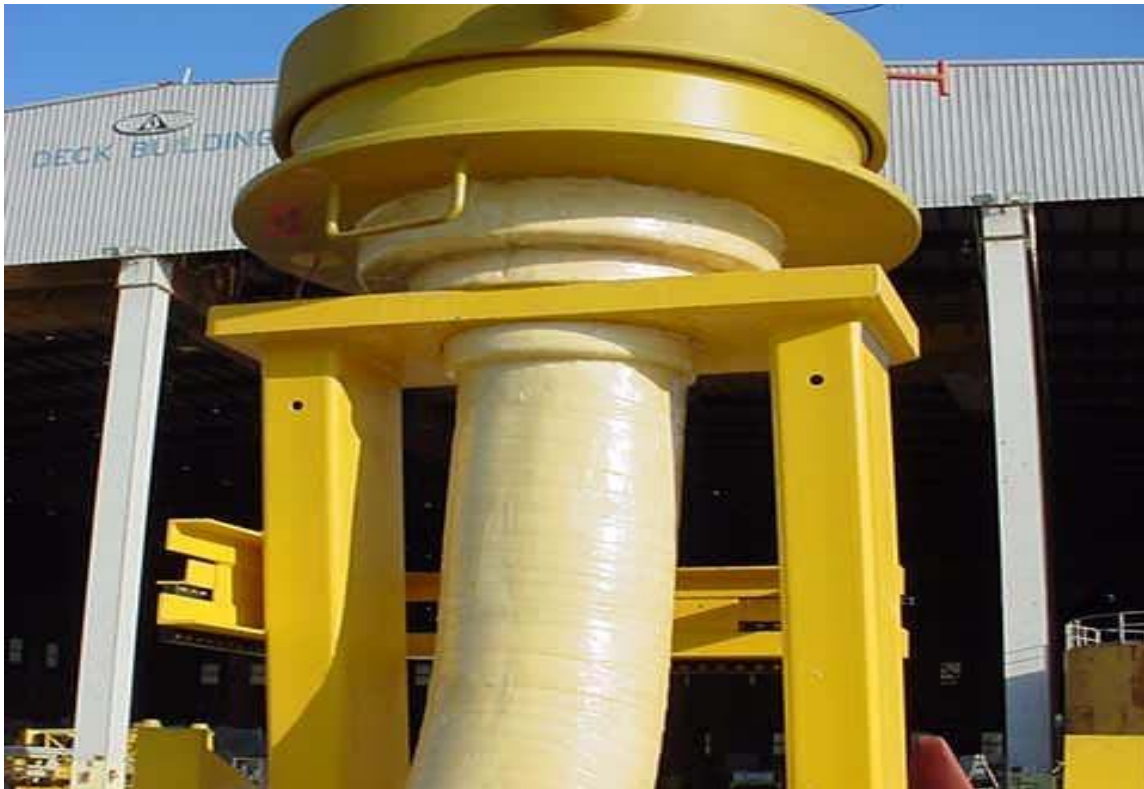
Figure 1. Epoxy Insulation Applied to Subsea Sled
