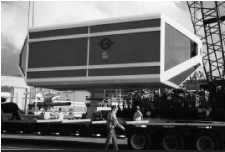
The Delmar buoys are rectangular with tapered ends for improved stability and handling. They include a central through-pipe for the in-line mooring chain with a stopper plate at each end for easy deployment and retrieval. A rugged outer steel cage provides impact and abrasion damage resistance.
