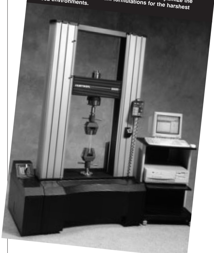
The Instron Universal Tensile Tester allows us to optimize the performance of syntactic foam formulations for the harshest subsea environments.
