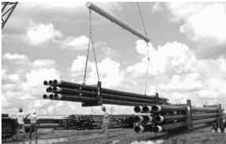
Kizomba riser joints in bolsters are loaded for shipment.
