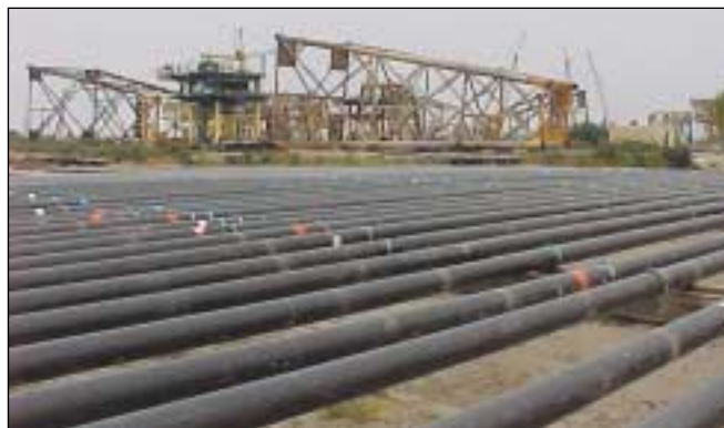
Syntactic foam can also be used as insulation on flowlines, such as these quad-joints for Shell Exploration & Production Inc.'s King development (Fig. 3).
