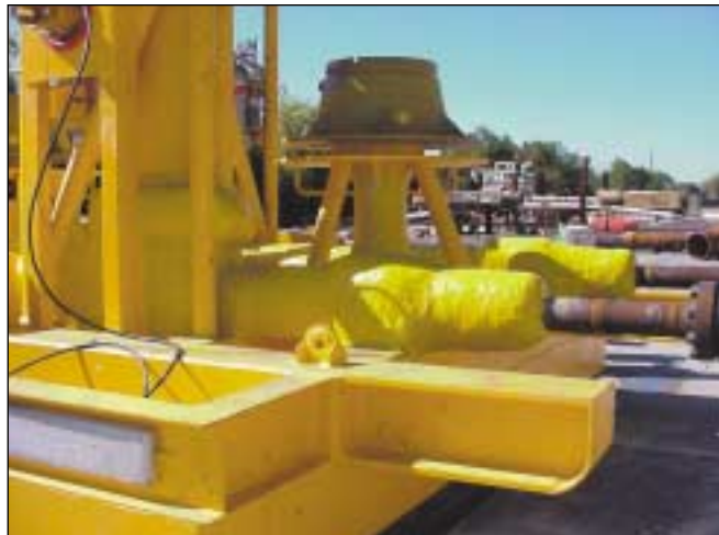
Syntactic foam insulates Shell Exploration & Production's King pipeline-end manifold (PLEM) (Fig. 2).
