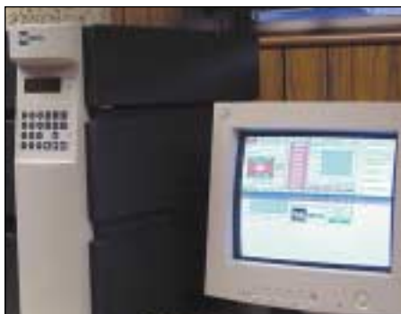
A holometrix cell is a typical thermal-conductivity measuring device (Fig. 4).
